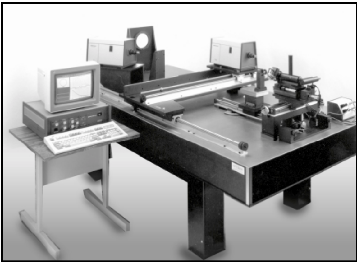
FIGURE 1. A typical MTF measurement instrument will allow full freedom to create a test environment exactly as the design environment, including spectral filtering, off-axis evaluation, conjugate matching, and image plane movement.
